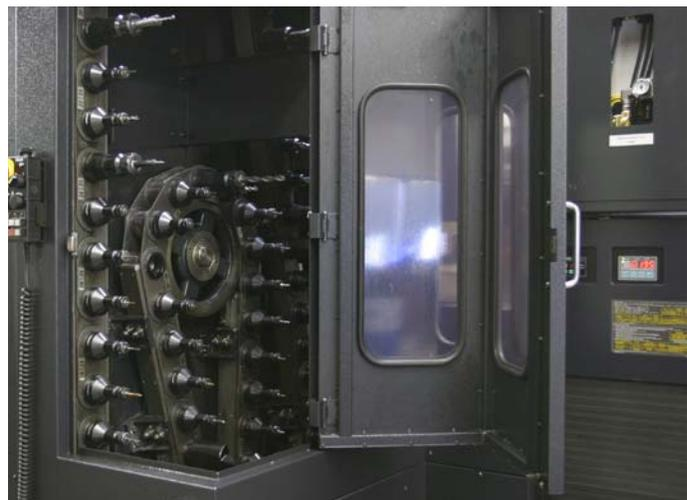
**View of the 120-tool turret on the Mazak Integrex.**
