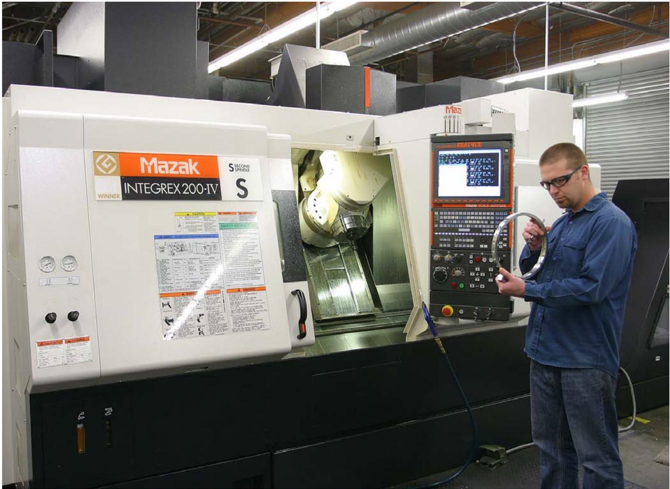
**Seth Larkin, lathe department manager, checks a part just completed on the Mazak Integrex 200-IV multi-tasking machining center. The Integrex has a 120-tool changer, dual spindles for milling and turning. Milling spindle is 12,000 rpm. Lathe spindle is 5,000 rpm.**
